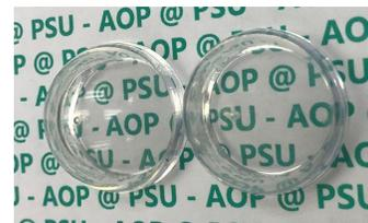
"This discovery came about as we were trying to make higher-efficiency solar panels," said Chris Giebink, associate professor of electrical engineering, Penn State. "Our approach involved concentrating light onto small, high-efficiency solar cells using plastic lenses, and we needed to minimize their reflection loss." >>
